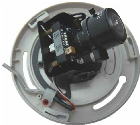
Advert AD-04 PRO With Vari-Focal lens and Top access DIP switch controls
